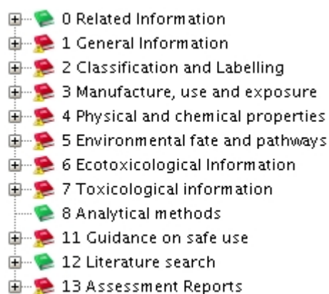
Picture 2. The structure of the REACH dossier in the IUCLID5 format.
