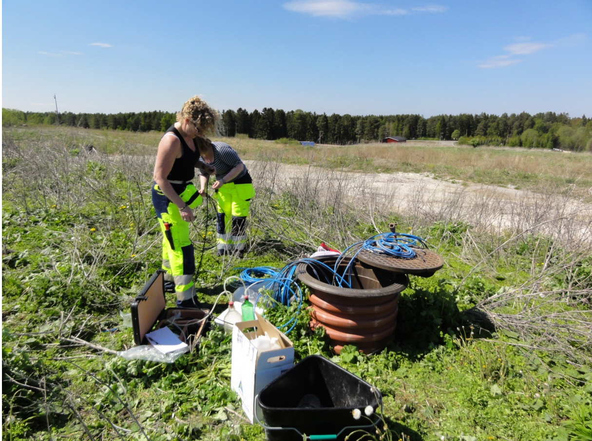
Picture 4 Pumping leachate from the lysimeters, using vacuum pump. The blue tubes are for water and the black for to let the air come in to the lysimeter. Just to avoid underpressure in the lysimeters.
